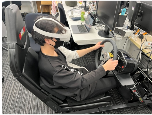
Figure 3: Data from the pedals and steering wheel and the participant's head motions in the real world are linked to the car's velocity and the view in the HMD.
